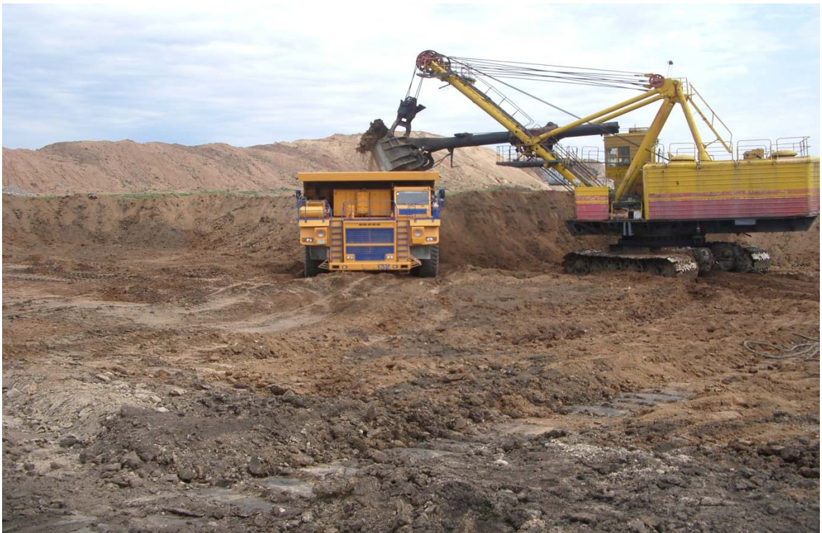
Fig. 2. The conditions of haulage in Tugnuisky mine. Belaz 75131 dump truck and EKG-12,5 (12,5 v3) rope shovel.
